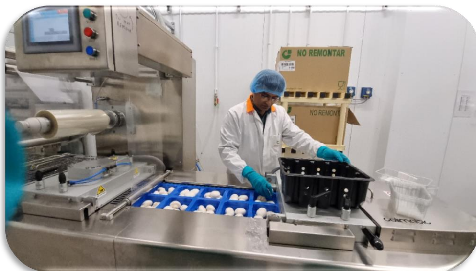
Plate HRD-4 : Packaging of fresh mushrooms using Thermosealer
