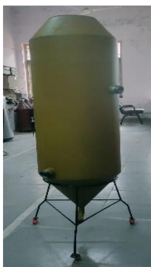
Plate. 4.1 : Fabricated silo bin for 100 kg wheat capacity
