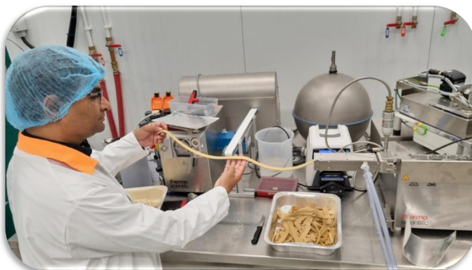
Plate HRD – 2 : Preparation of high moisture meat analogue from protein isolates
