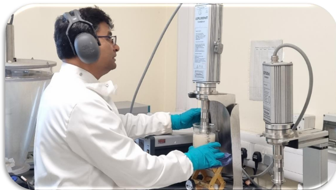
Plate HRD – 3 : Extraction of chitosan using Ultrasound technology
